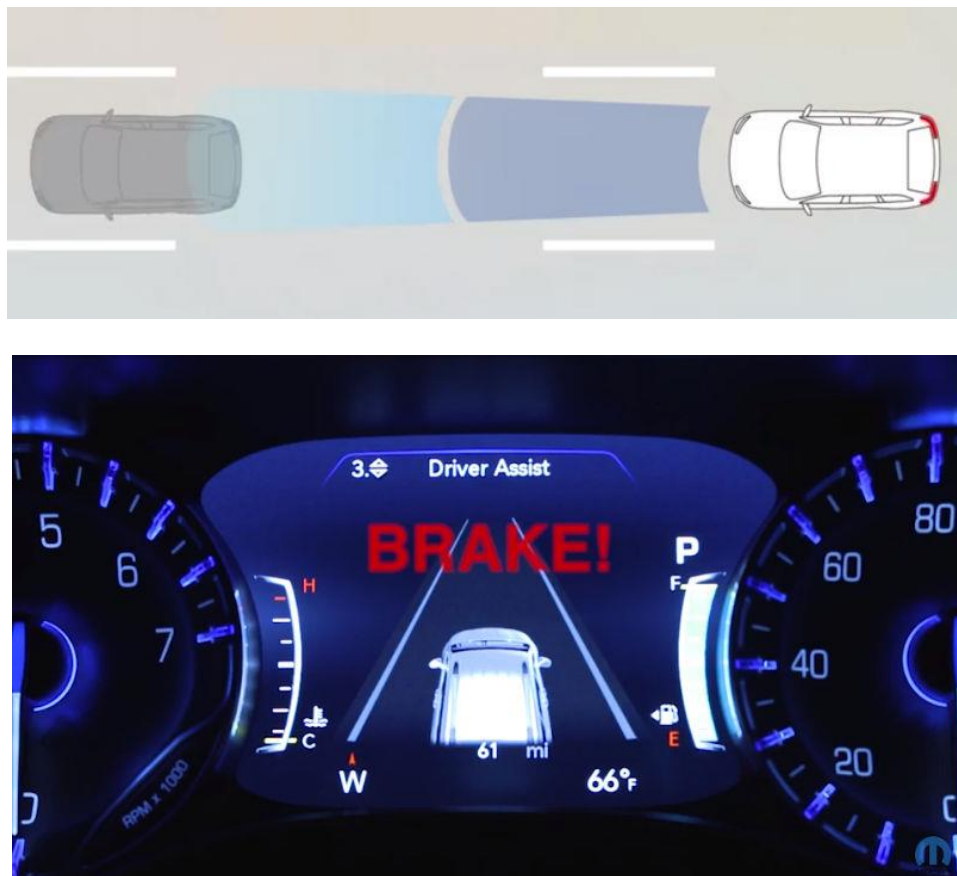
Figure 1. Operation of Forward Collision Warning System
