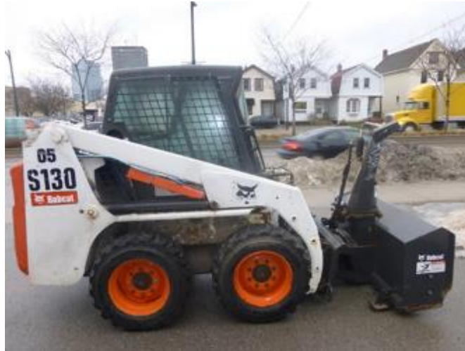
Bobcat S130 skid-steer loader equipped with a blower (Source: TSB)
